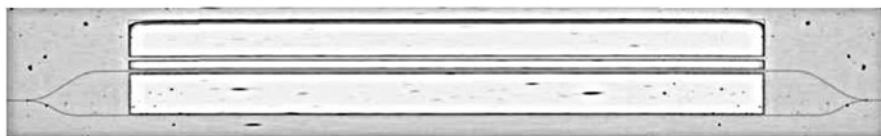
Fig. 9.16 Asymmetric Mach – Zehnder interferometer with the active region localized in both arms
